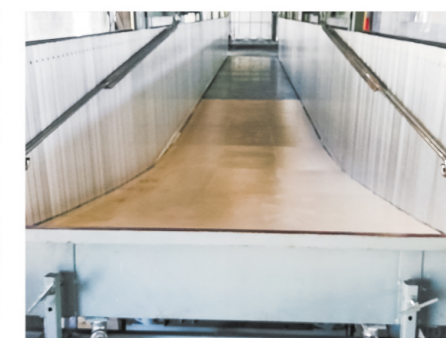
溢流槽 Overflow trough
